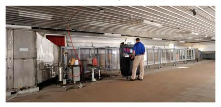
The spray is analyzed using a laser refraction technology that measures drop sizes of the spray coming out of a nozzle. The data that is generated is typically expressed as either the number of drops less than 105 microns, or Dv 10 which is the drop diameter where 10% of drops are smaller and 90% of the drops are larger. The larger the Dv10, the less prone the spray will be to produce drift prone droplets.
