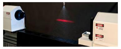
Accomplice and leading DRAs were tested at the University of Nebraska, Pesticide Application Technology Lab in North Platte, Nebraska using low wind speed (16 mph) and high wind speed (125 mph), to simulate ground and aerial spray applications, respectively. Two broad spectrum herbicides were tank mixed with Accomplice and the leading DRAs.
